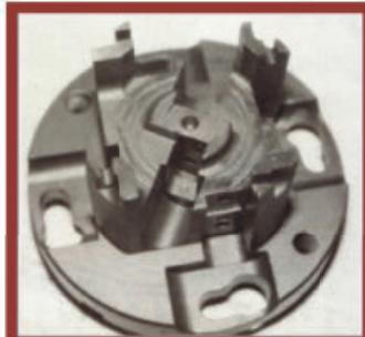
Hollow Mill for Turning, Facing,
