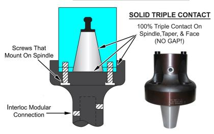
Interloc Rigid MFH holders will fit most standard bolt down machine spindle heads & have a tapered plug available in CAT-50 or CAT-50 NMTB.
